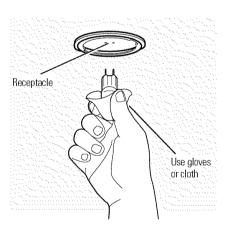
Push the bulb straight into the 3 receptacle all the way.
