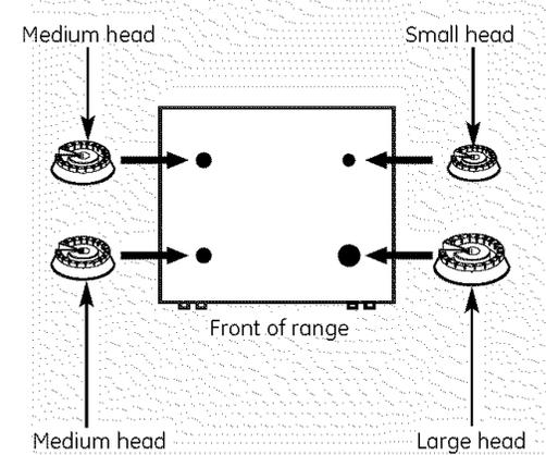
Make sure the slot in the burner head is positioned over the electrode.
