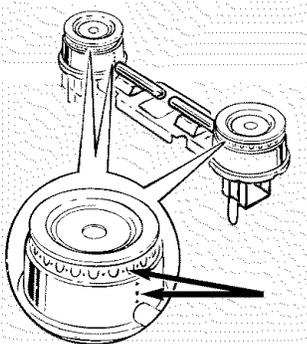
Check the flame pattern of each burner. If the flames are “jumpy” (not steady), clean the holes again with a sewing needle or twist-tie.
