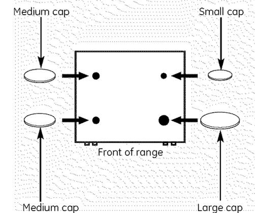
Make sure that the heads and caps are replaced in the correct locations.
