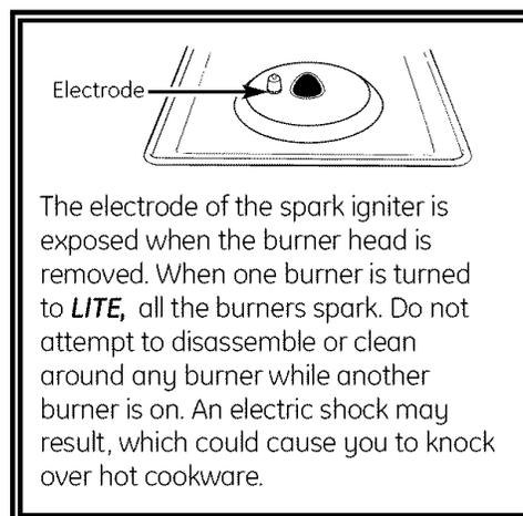
The electrode of the spark igniter is exposed when the burner head is removed. When one burner is turned to **LITE**, all the burners spark. Do not attempt to disassemble or clean around any burner while another burner is on. An electric shock may result, which could cause you to knock over hot cookware.
