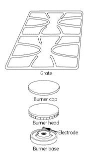
**CAUTION:** Do not operate the burner without all burner parts in place.
