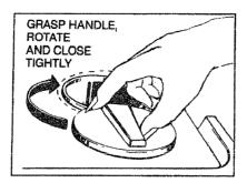
Always close the main cup tightly. When it is firmly latched you will hear a clicking sound. It is not necessary to overtighten.
