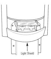
**A**WARNING – The light shield must be replaced or the heat from the bulb could damage the refrigerator.
