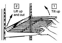
To relocate shelves: Select desired shelf height. With shelf front raised slightly, engage the top lugs in the tracks at the rear of the cabinet. Then lower the front of the shelf until it locks into position.
