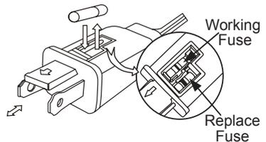
**WARNING:** **Risk of Fire:** Do not replace the attachment plug. Contains a safety device (fuse) that should not be removed. Discard product if attachment plug is damaged.
