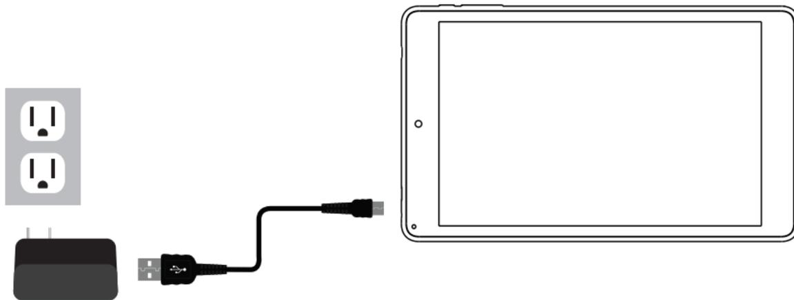
Connect the power adapter to a wall outlet, then to the tablet's micro USB port as shown. It is recommended to fully charge the battery before first use. A battery status indicator appears in the lower right corner of the Task Bar. Tap to view the current battery level, time remaining, brightness control, and settings for power and sleep modes.
