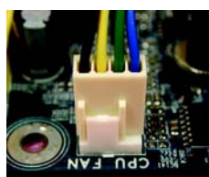
Fig. 6 Finally, please attach the power connector of the heatsink to the CPU fan header located on the motherboard.
