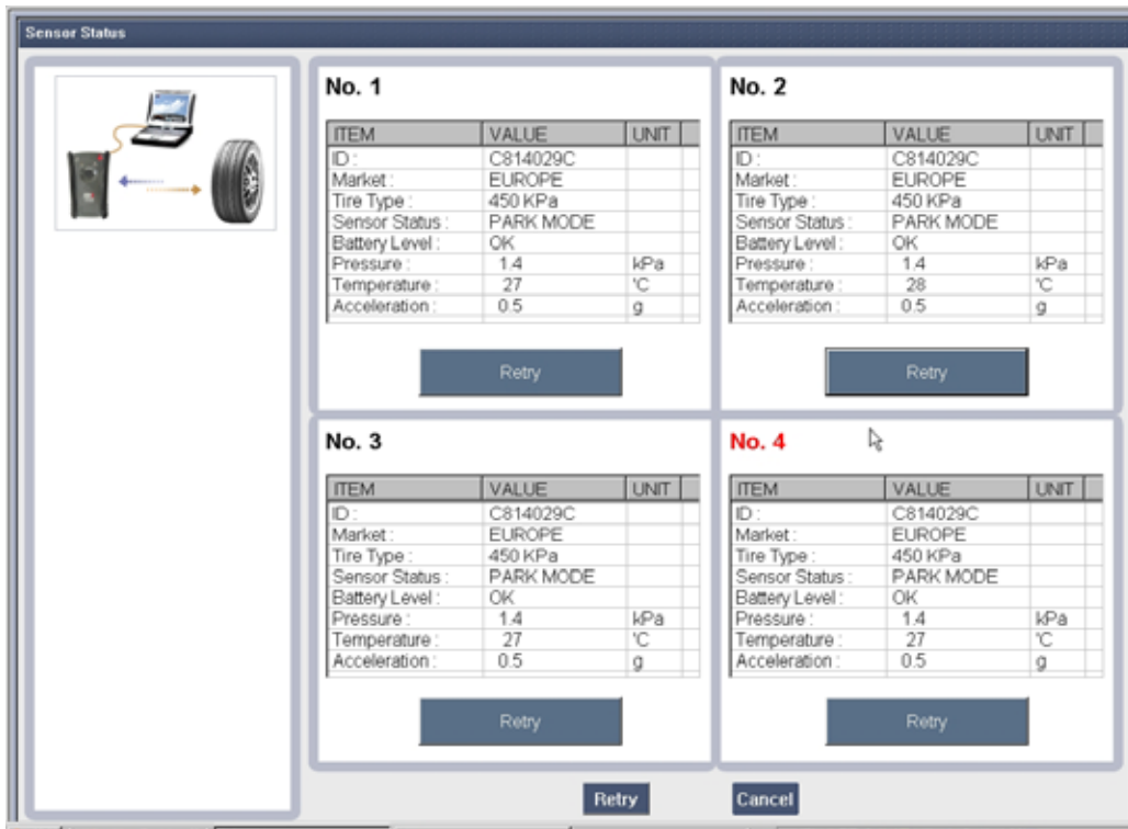
< Figure 1-3. Sensor Status Checking >
