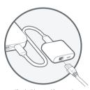
Plug the Ethernet cable connecting to your computer into the LAN port of the USB-C port replicator
