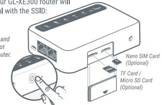
After inserting cards, turn on the router by pressing the power button
