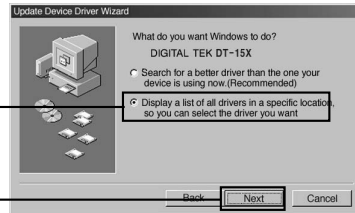
8 Click "Display a list of all the drivers in a specific location, so you can select the driver you want"
