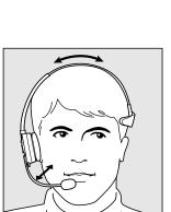
To change or clean the ear cushion, first remove the 30 earplate by turning the earplate 45 degrees counterclockwise. Once removed, the ear cushion can be taken off the earplate.
