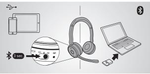
Hold the Bluetooth switch for 3 seconds. Wear the headset and follow the voice-guided pairing instructions. Insert the USB dongle into your PC. The headset and the USB dongle are pre-paired.
