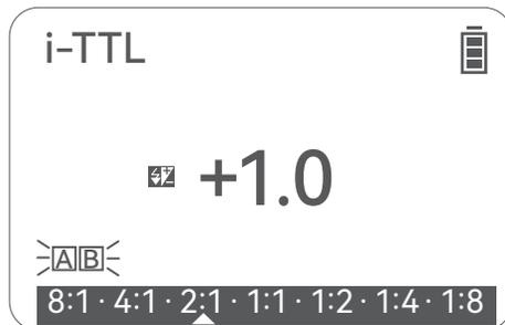
Short press the SET button to select <FEB> > FEB/A:B flash ratio, turn the select dial to adjust the FEB/A:B flash ratio. The FEB value is adjustable from -3 to +3 with an increment of 1/3 each stop, while A:B flash ratio is adjustable from 8:1 to 1:8 with an increment of 1/2 each stop (for example: 8:1 5.6:1 4:1 2.8:1 2:1 1.4:1 1:1 1:1.4 1:2 1:2.8 1:4 1:5.6 1:8).
