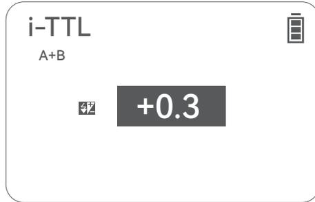
Turn the select dial to adjust the FEB value from -3 to +3 with an increment of 1/3 each stop.
