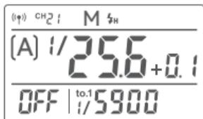
3. Connect the studio flash to power source and power it on. Press the MODE/Wireless button to make the < (A) > displayed on the panel and enter 2.4GHz wireless mode. Press and hold the <GR/CH> button to set the same channel to the flash trigger, and press the < GR/CH > button to set the same group to the flash trigger.
