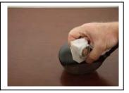
Once the club head module is removed, the remaining tape must be removed from the club head. One method is to roll the tape off of the club head with your thumb, which is the safest way to remove the tape with out damaging the club head paint.
