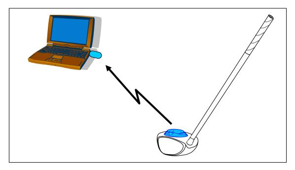
Once the computer receives the data, the "User Application" software processes that data instantaneously into useful information for presentation to the golfer through a rich graphics interface on the computer screen.
