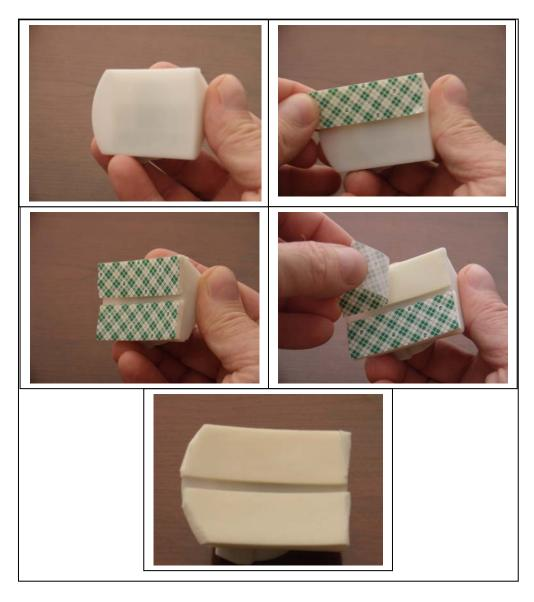
Align the front of the Club Head Module parallel with the club face and align about  $\frac{1}{2}$  inch back from the club face and firmly press the module onto the club head as shown below. The double sided adhesive tape is the 3M 4008 tape which is  $\frac{1}{8}$  thick.
