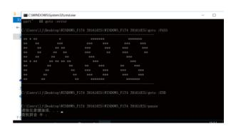
Step 5: Restart the device (do not to plug in the charger at this time, otherwise the charging screen will pop up. You can press Ctrl + Alt + Del to restart). The screen will turn black for about 1 minute after restart, then the BIOS will reboot twice for automatic updating purposes, never do forced shutdown at this time!
