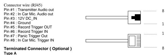
1) Wire the un-terminated signal wires to the control unit according to the signal chart. 5 Amp fast blow fuse is recommend in the 12VDC power supply line to protect the equipment.
