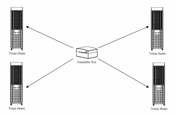
In the broadcasting mode, one Transmitter Box can be connected to 50 Heaters.
