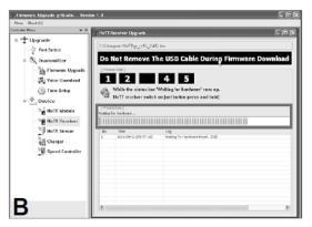
Start the SJ Firmware Update Utility and select the correct COM port, "Silicon Labs CP210x USB to UART Bridge", at [Port Select]. Choose the "HSTT receiver update" menu. After clicking the "File Browse" button, find and select the firmware file with extension "bin" from the folder. Now click "Program" button and wait briefly until you see movement in the progress bar. It may take about 5 sec, depending on the computer.
