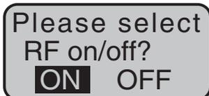
After the transmitter is switched on by fixed wing of type "Motor on C1 front/rear" the position of the output 1, so as in heli model the output 6 connected servo, will be verified. If the related servo is out of the idle position and because of the danger connected to a rotating motor, the RF module remains off for safety reasons.
