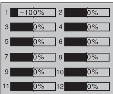
Otherwise the graph bars show current setting percentages for control stick control functions which are not self-neutralizing.
