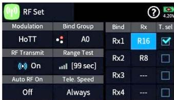
Up to four receivers can be bound to each model memory in the submenu “RF Set”. However, a telemetry connection can only be established to one of these four receivers. The standard telemetry receiver is always the last one bound.
