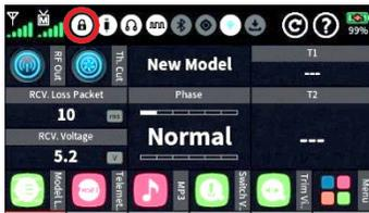
In the basic display of the transmitter, the input lock of the screen is activated by pressing the two lower selection keys simultaneously for approx. 1 second.
