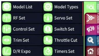
Touching the "Menu" field at the bottom right of the main display changes to the last tab of the four tabs or menu lists labeled "Basic", "Function", "Special" and "System".
