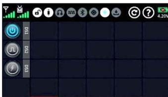
The mz-32 HoTT transmitter features 64 digital switches. These can be found in the “Special” menu and can be defined, activated and switched in the submenu “Digital Switch”. In addition, each of these 64 Digital Switches can be arbitrarily placed as a widget on one of the widget pages and operated from there.
