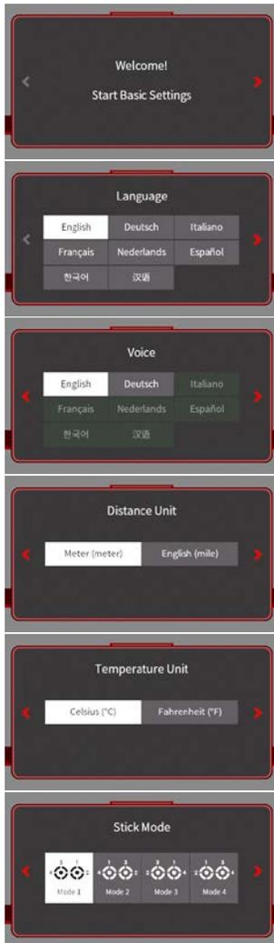
If the transmitter is still in the delivery status or the transmitter was previously reset to factory settings in the "Info & Update" menu, an almost self-explanatory wizard starts immediately after the transmitter is switched on to obtain user settings preferences.
