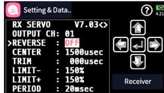
This display visualizes the settings and menus of the connected receiver. If there is no connection to a receiver, the submenu can be opened, but the display window remains empty.
