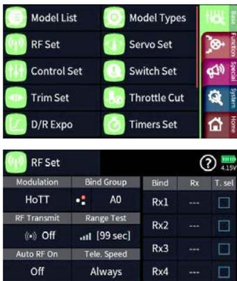
If the bind was successful you will notice in the Rx column of the transmitter the number of receiver channels for example R6, R12 with a highlighted blue background and the LED on the receiver will change its color or state.
