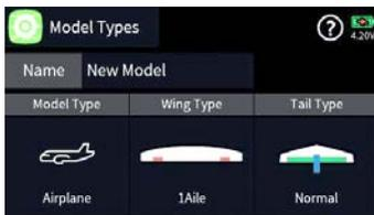
Tapping a menu opens the corresponding menu, for example the submenu "Model Type".
