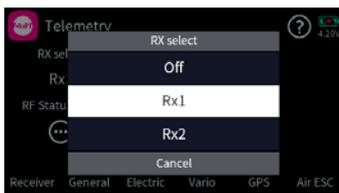
In the “RF Set” menu the receiver that has the “T.Sel” field checked is the receiver that provides telemetric information to the transmitter
