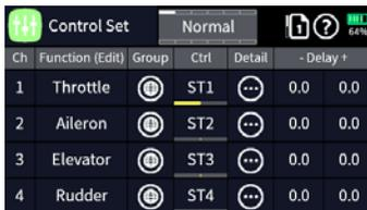
2. On the desired channel touch the detail icon in the “Detail” column for example, throttle.
