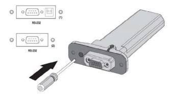
1. If the RS232 port is compliant with the specification (1), please turn on the DIP switch, then plug the Bluetooth Module to the inverter directly via the RS232 and lock screw.
