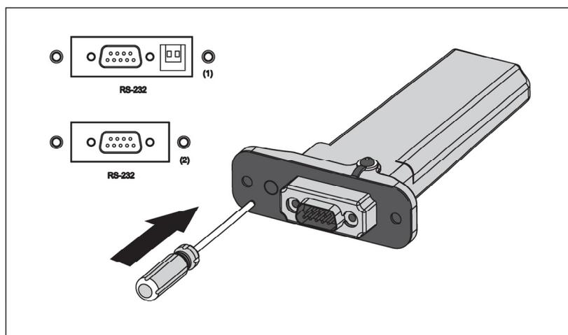
Wi-Fi Module is connected to inverter via RS232. Plug Wi-Fi module into inverter, and lock screw.
