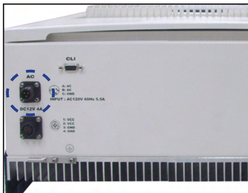
<Figure 9> AC Power Port Connection
