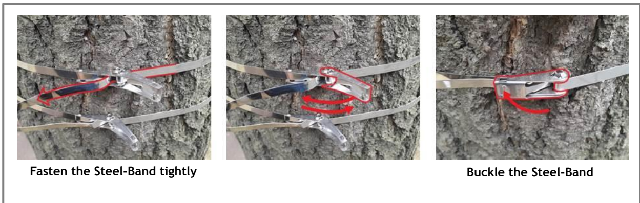
Figure 16. The way to using a Steel Band
