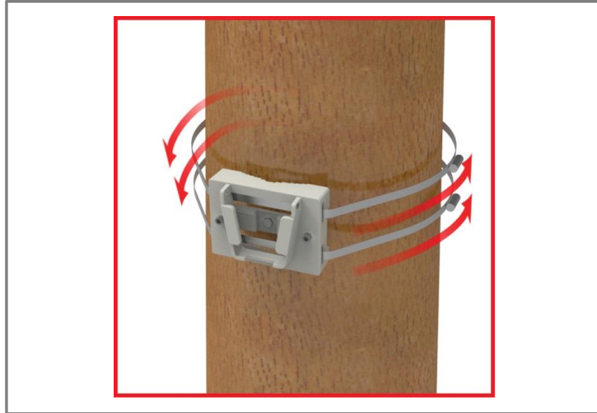
Figure 15. Installing the Steel Band
