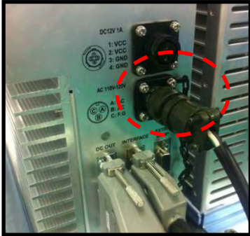
<Picture 10> AC Power Port Connection.
