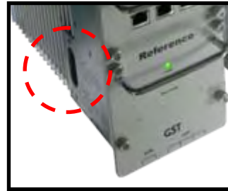
<Picture 11> ON/OFF Switch of SpeedCell Repeater.
