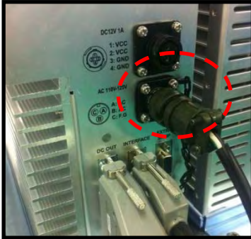
<Picture 10> AC Power Port Connection.
