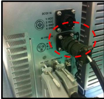
<Picture 10> AC Power Port Connection.
