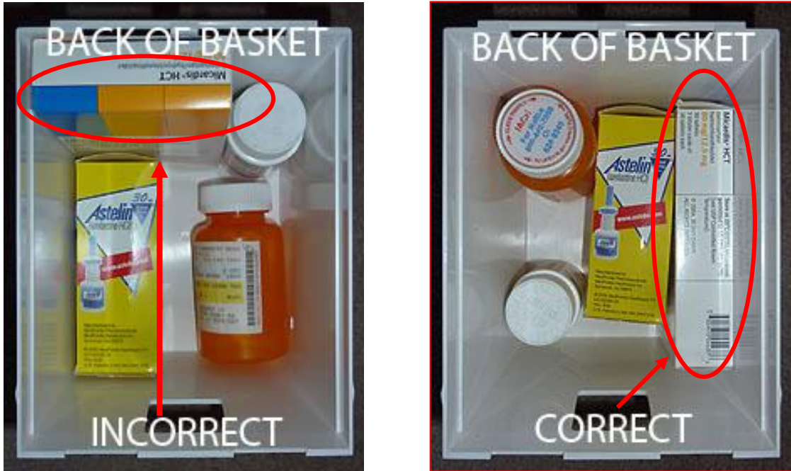
Figures 11 and 12. Incorrect and Correct placement of items in SmartBasket. Foil packaging should not be placed at back of basket.
