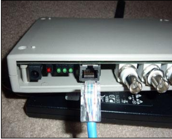
Figure 73. Front of RFID Reader with Ethernet cable.
