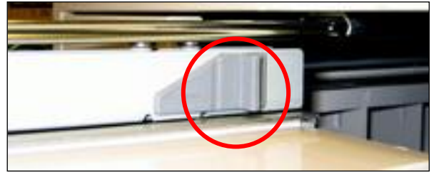
Figure 65. Slide extension stop.
