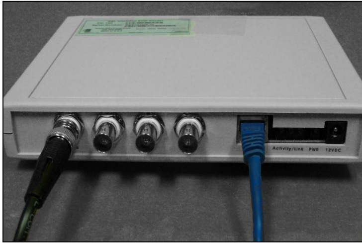
Figure 75. Coaxial Cable is attached to connector on left side.
