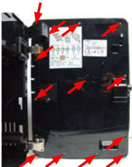
Loosen the screws as shown to remove the inner cover of the front panel and disconnect the electrical connections
