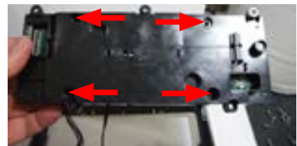
Loosen the screws as shown and remove the cover
