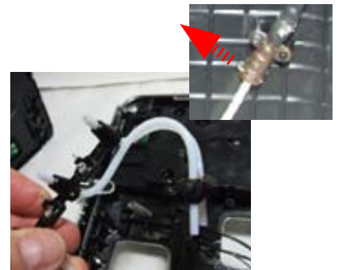
Disconnect the pipe from the Teflon by removing the fork and remove the Teflon pipe support assembly
