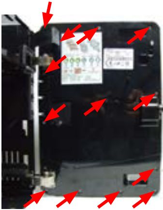
Loosen the screws as shown to remove the inner cover of the front panel
