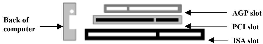
AGP vs. PCI vs. ISA expansion slots
