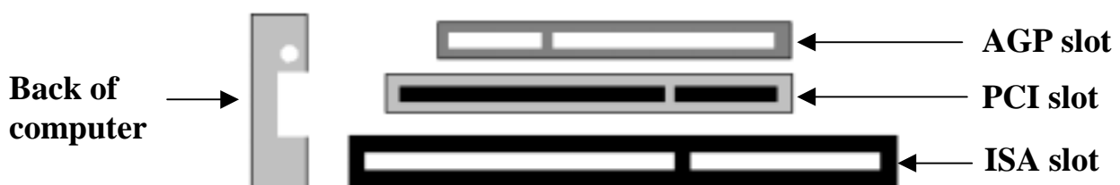
AGP vs. PCI vs. ISA expansion slots
