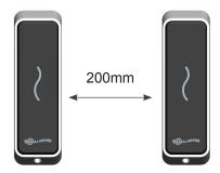
When mounting a proximity reader on an internal wall, check that any reader fixed to the other side of the wall is not less than 200mm (8 inches) away.
