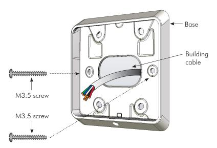
4. Connect the reader tail extending from the facia assembly to the building cable. Connect the wires shown below.
