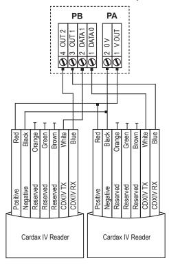
Note: Within each group, you cannot mix Cardax IV readers with Wiegand Readers. This is because connecting one Wiegand reader requires all four pins on plug PB. For example, if you connect a Cardax IV reader to Port 1 of Group 1, Port 2 of Group 1 can only connect to another Cardax IV reader.
