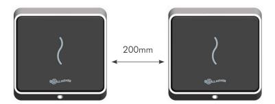
When mounting a proximity reader on an internal wall, check that any reader fixed to the other side of the wall is not less than 200mm (8 inches) away.
