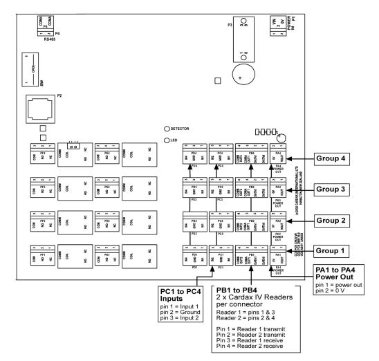
Make the connections from the Gallagher T12 Reader to either the Cardax FT Controller 3000-4R or 3000-8R as shown:
