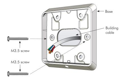
4. Connect the reader tail extending from the facia assembly to the building cable. Connect the wires shown below.
