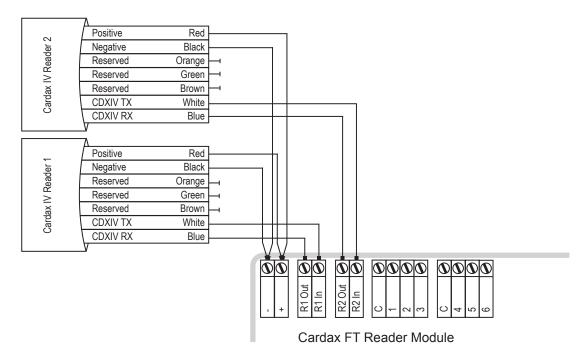
Connect the wires to the sockets as shown:
