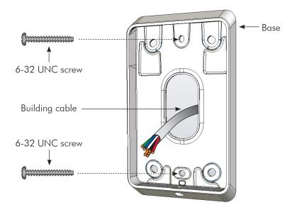
4. Connect the reader tail extending from the facia assembly to the building cable. Connect the wires shown below.
