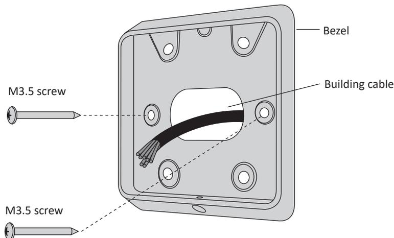
4. Connect the reader tail extending from the facia assembly to the building cable. Connect the wires for the appropriate reader you wish to interface, either an HBUS Reader or a Cardax IV Reader, as shown in the following diagrams.
