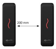
When mounting a proximity reader on an internal wall, check that any reader fixed to the other side of the wall is not less than 200 mm (8 inches) away.
