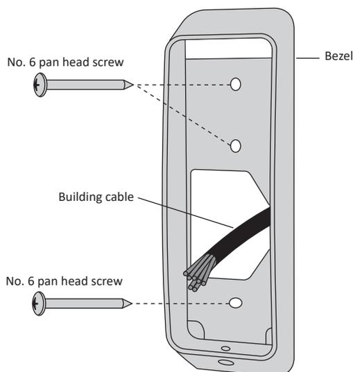
4. Connect the reader tail extending from the facia assembly to the building cable. Connect the wires for the appropriate reader you wish to interface, either an HBUS Reader or a Cardax IV Reader, as shown in the following diagrams.
