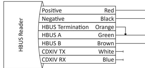
**Note:** To terminate an HBUS Reader, connect the **Orange** (HBUS Termination) wire to the **Green** (HBUS A) wire.
