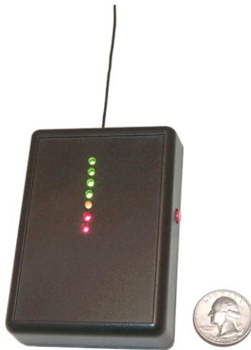
Figure 3. Handheld Signal Strength Meter (SSM)
