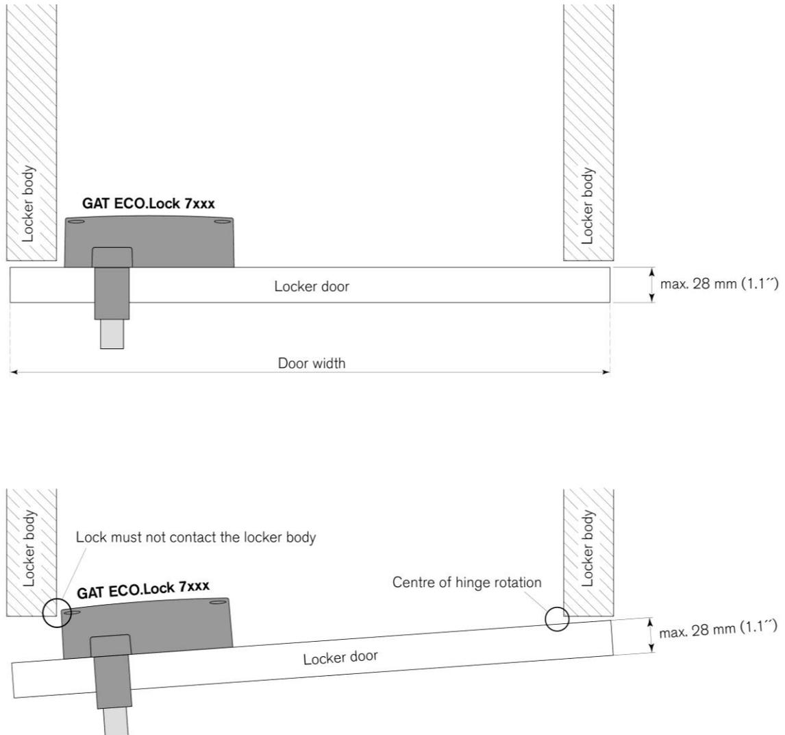
Figure 3.1 – Width and thickness of the locker door
