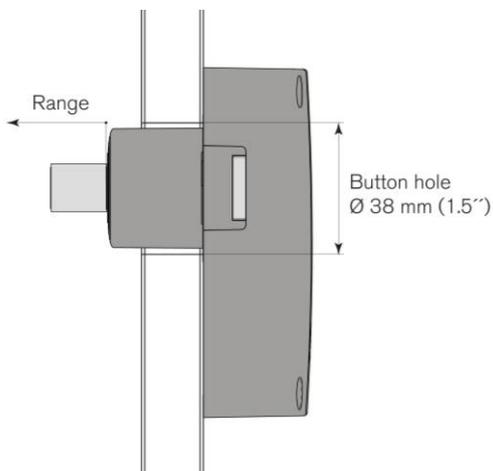
Figure 3.7 – Diameter of the button drill hole for metallic doors
