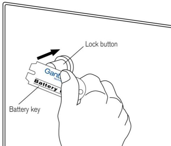
**Figure 4.3** – Activating the GAT ECO.Lock 7xxx F/ISO with the battery cover key
