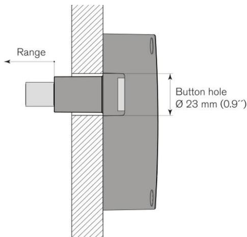
**Figure 3.3** – Diameter of the button drill hole for non-metallic doors
