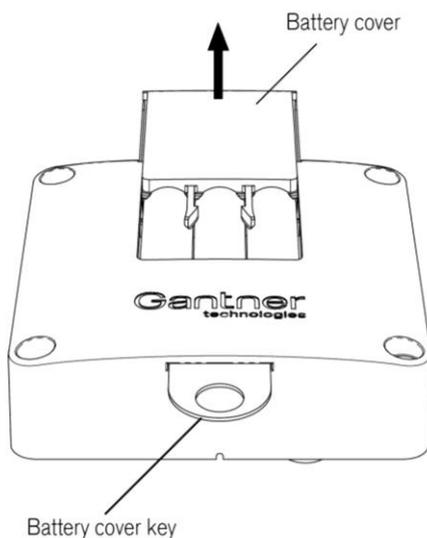
**Figure 4.1** - GAT ECO.Lock 7xxx F/ISO battery compartment
