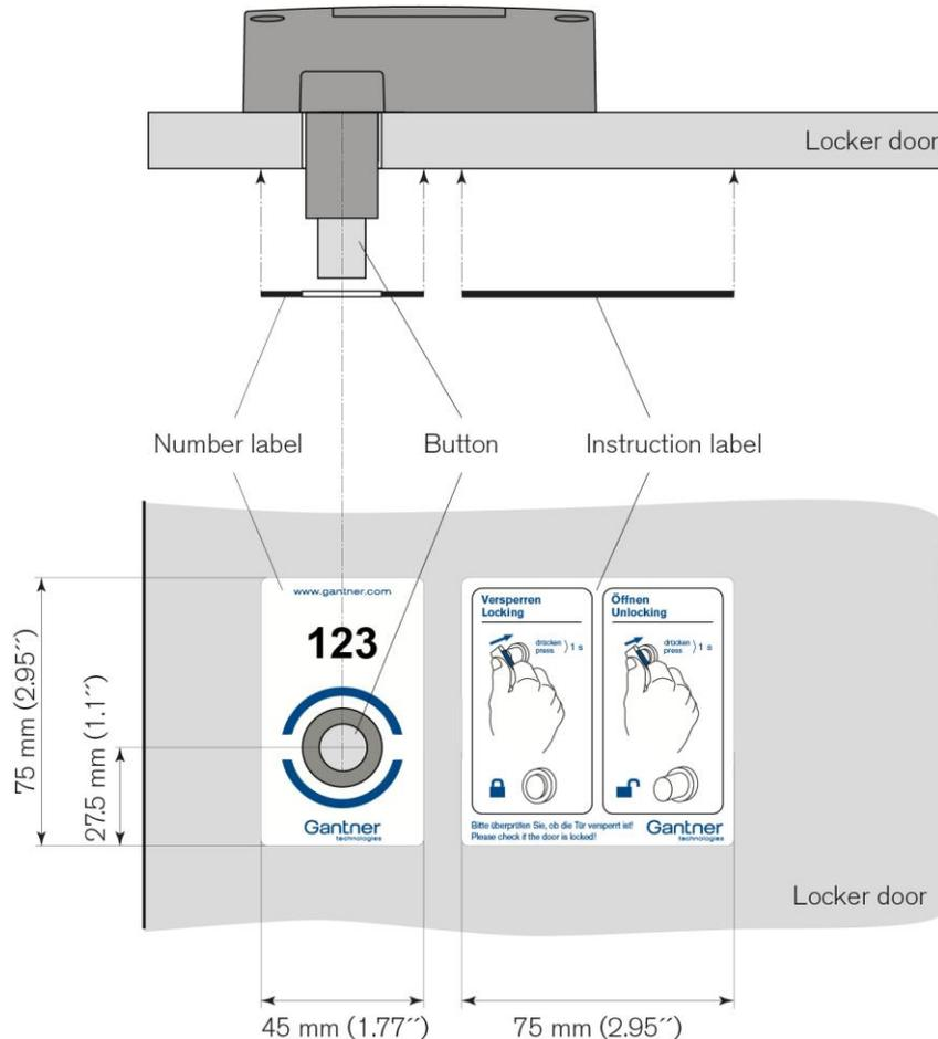
**Figure 3.11** – Label attachment for a right-hinged door
