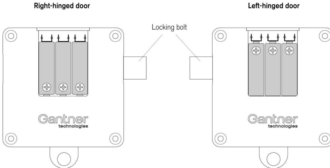
**Figure 4.2** – Correct battery polarity
