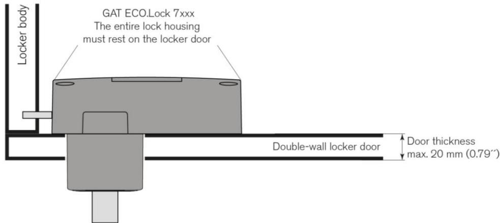
**Figure 3.10** – Installation of the GAT ECO.Lock 7xxx F/ISO on a double-wall metallic door
