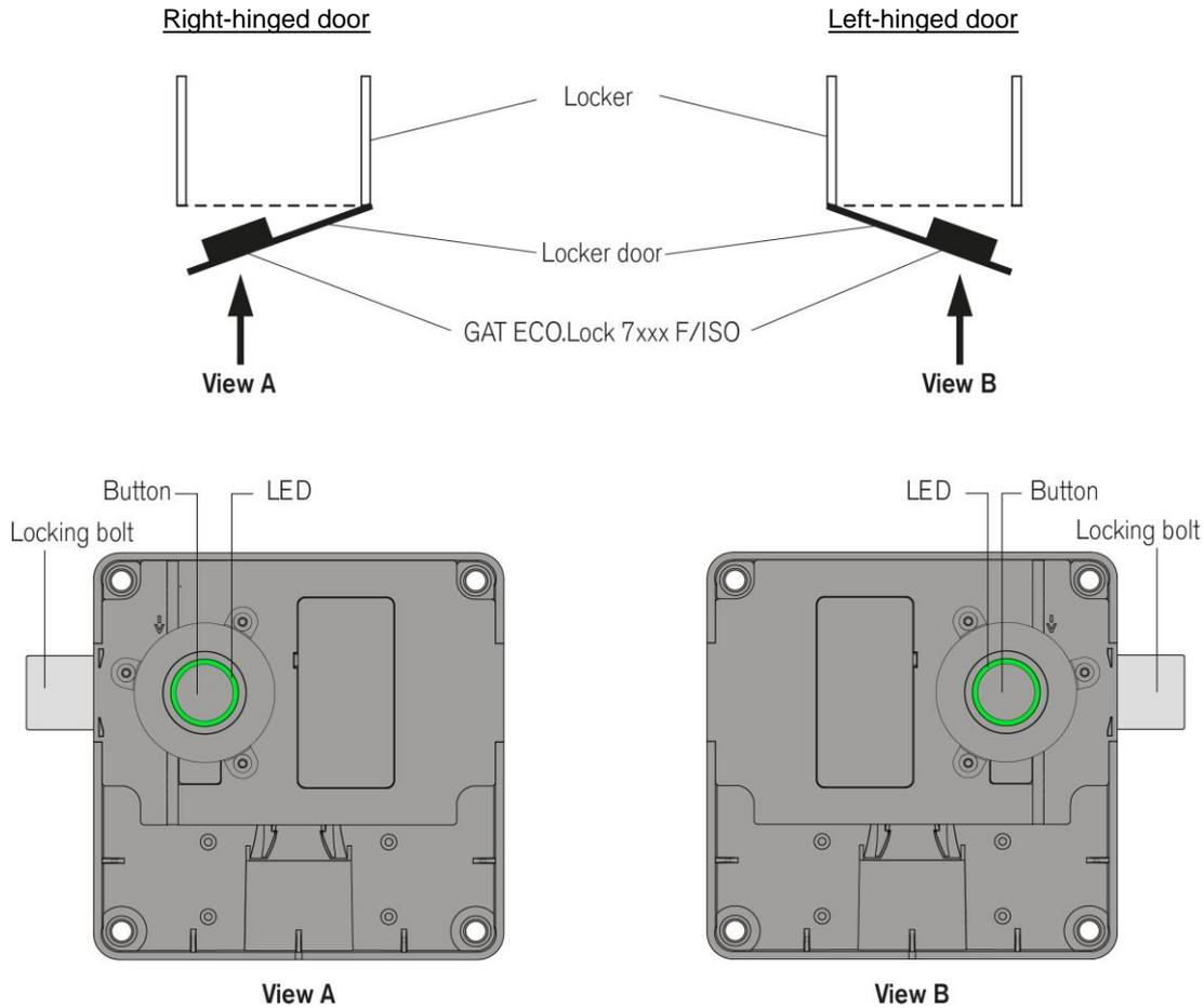
**Figure 3.2** – Locker door hinge definition (left/right)
