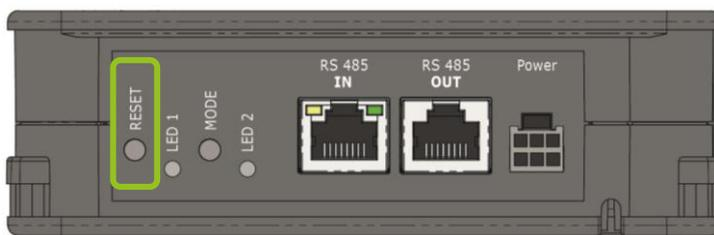
Figure 5.2 – RESET button for restarting a controller (sub controller shown)
