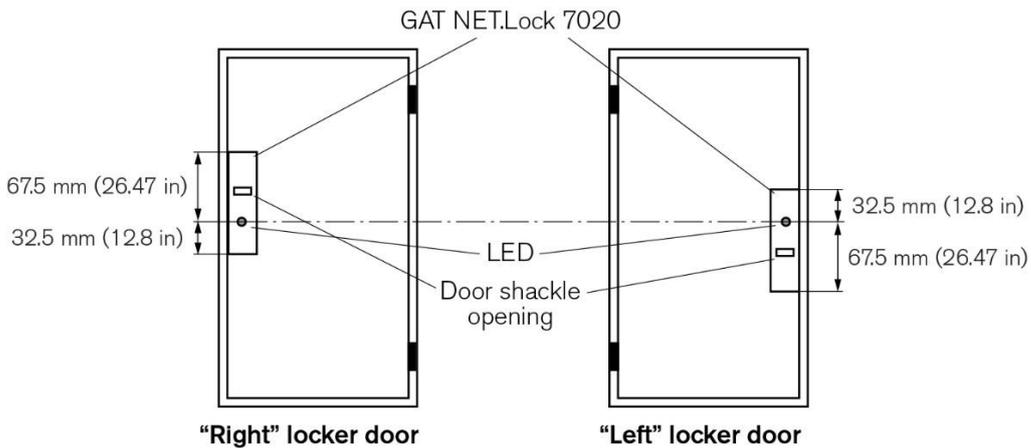
Figure 3.1 - Definition of the opening direction of lockers (left/right)
