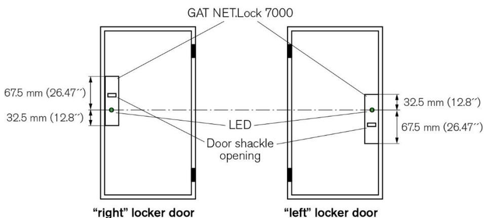
**Figure 3.2** - LED positions of the GAT NET.Lock 7020 for right and left-hinged doors
