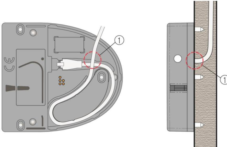
**Figure 4.3** - GAT NET.Lock 7020 cable routing
