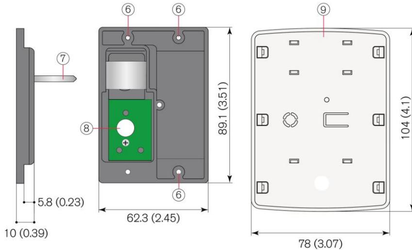
**Figure 3.7** - Dimensions of the GAT NET.Lock BoltSet 7220
