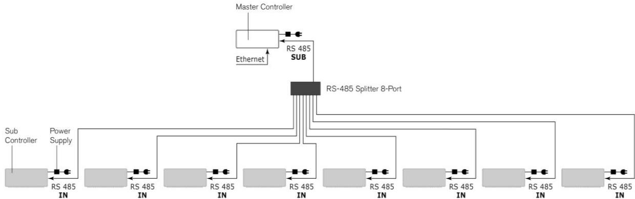
**Figure 4.8** – Parallel connection of the GAT NET.Controller S 7020
