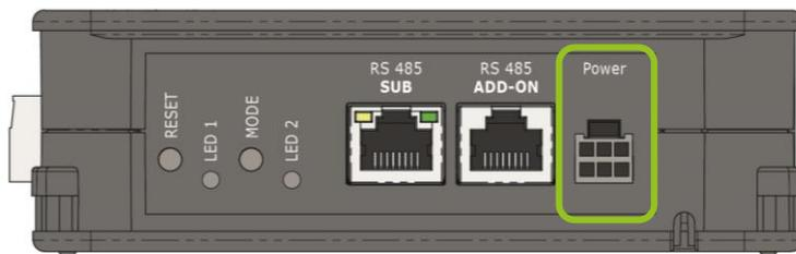
Figure 4.13 - Power supply connection on the GAT NET.Controller M 7020
