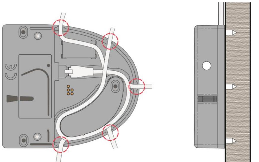
Figure 4.2 - GAT NET.Lock 7020 cable outlets
