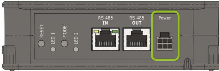
**Figure 4.10** - Power supply connection on the GAT NET.Controller S 7020
