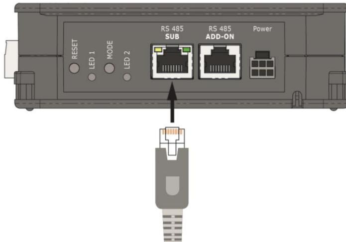
Figure 4.9 – Connecting the GAT NET.Controller S 7020 to the GAT NET.Controller M 7020
