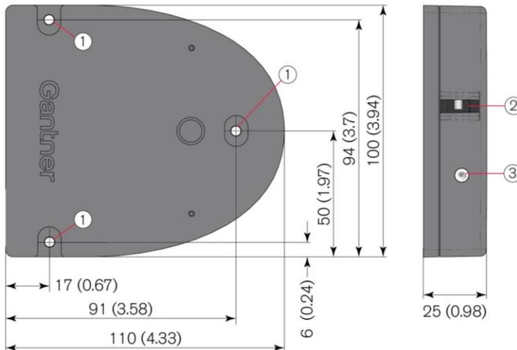
Figure 3.4 - Dimensions of the GAT NET.Lock 7020 / GAT NET.Lock 7020 P
