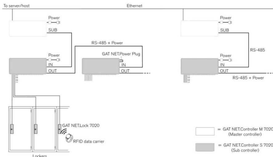
Figure 4.1 - GAT NET.Lock 7020 system structure
