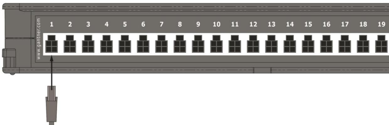
Figure 4.4 – Connecting the GAT NET.Lock 7020 to a GAT NET.Controller S 7020 sub controller
