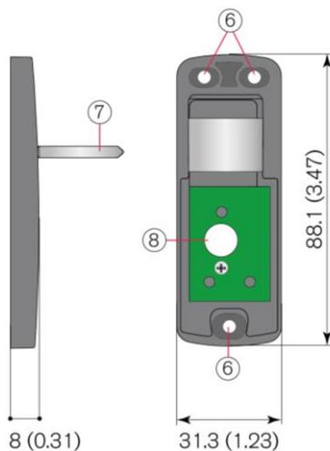
**Figure 3.6** - Dimensions of the GAT NET.Lock BoltSet 7120
