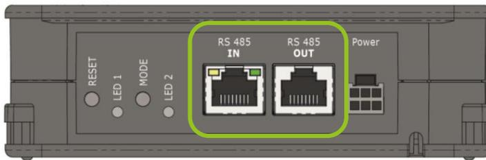
Figure 4.5 – RS-485 connection on the GAT NET.Controller S 7020
