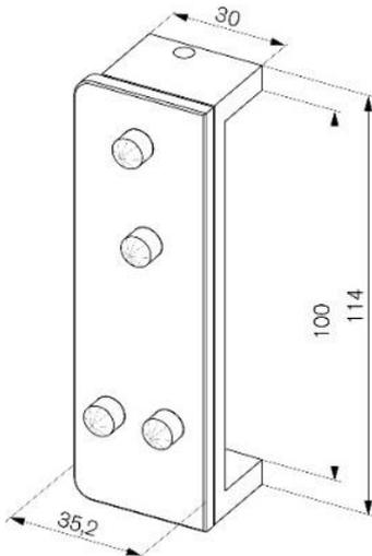
**Figure 3.3** – Bolt gauge (dimensions in mm)
