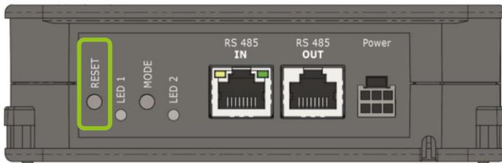
**Figure 5.3** – RESET button for resetting a controller (Sub controller shown)
