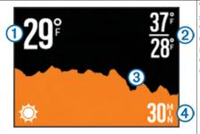
When connected to a sensor, tempe displays the current temperature ①, maximum and minimum temperatures ②, temperature graph ③, and time scale ④.
