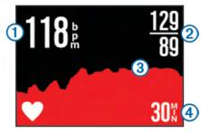
When connected to a sensor, heart rate displays the current heart rate ①, maximum and minimum heart rates ②, heart rate graph ③, and time scale ④.
