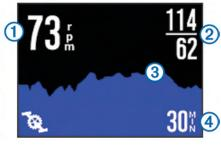
When connected to a sensor, cadence displays the current cadence ①, maximum and minimum cadences ②, cadence graph ③, and time scale ④.
