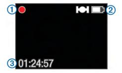
The viewfinder displays the recording status ①, the GPS and battery status ②, and the elapsed recording time ③.
