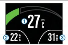
Speed displays the current speed ①, average speed ②, and maximum speed ③.
