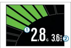
G-force displays the current g-force acceleration ① and maximum g-force acceleration ②.
