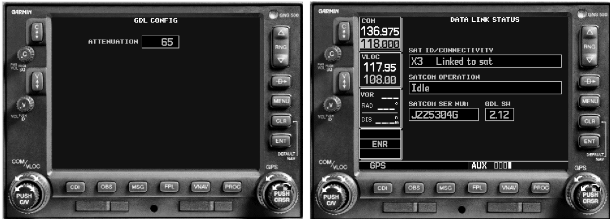
Figure 4-3. Data Link Configuration Page on the 400/500 Series (500 Series shown, 400 Series screen is similar)
