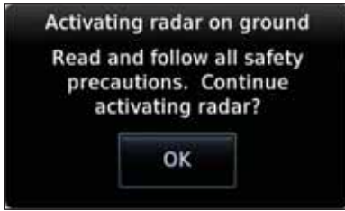
Figure 12-61 Caution for Radar Activation Confirmation
