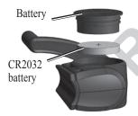
Use a coin to twist the cover counter-clockwise until it is loose enough to remove (arrow points to unlocked).
